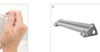
Place E-TRACK at desired location and Snap support stands onto the rear of E-TRACK. Refer to step 2 for positions of support stands.
