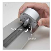
Align locator to V-Groove as shown and insert adaptor.
