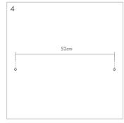
Measure and mark the locations for drilled holes as shown at the desired wall-mount location of E-TRACK. Use a levelling tool if necessary.
