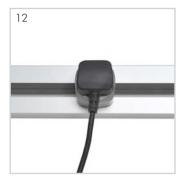
Insert plug and turn clockwise to engage power.
