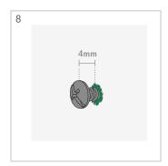
Fasten screws onto the wall plugs. Leave a gap of 4mm between the screw head and the wall surface for mounting.
