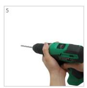
Drill holes on the markings made in step 3. Concrete Drill bit Ø 5.5mm.
