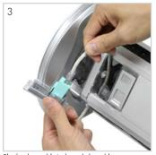
Slot the data cable in through the cable management compartment and insert the cable firmly into the rear of the data jack until it dicks.
